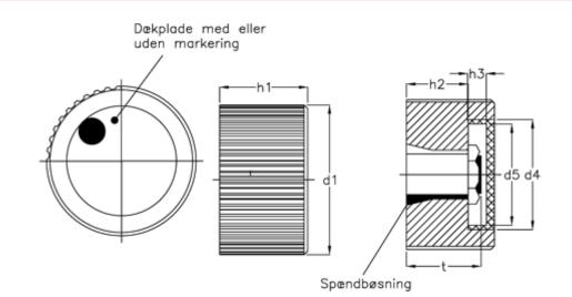
$\begin{array}{ll} d1 &= 27 \\ d3 &= Z6 \\ d4 &= 20 \\ d5 &= 18 \\ h1 &= 17 \\ h2 &= 11 \\ h3 &= 4.3 \\ t \ min = 14 \end{array}$
